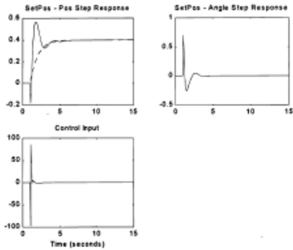
Fig. 7. Step responses of the cart position and of the rod angle with control input
