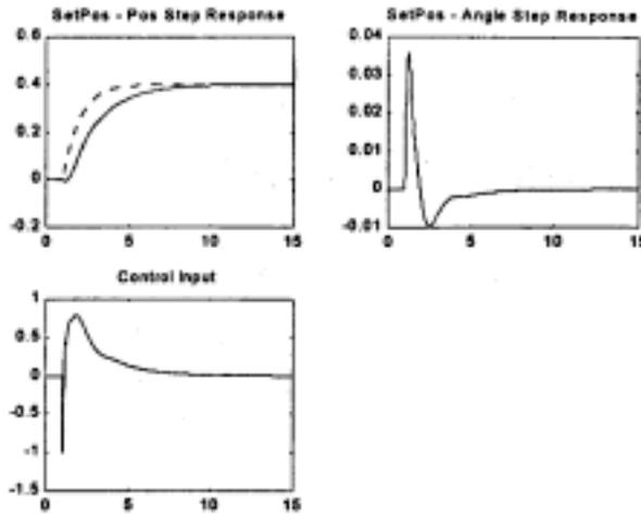
Fig. 11. Step responses of the position and of the angle with control input
