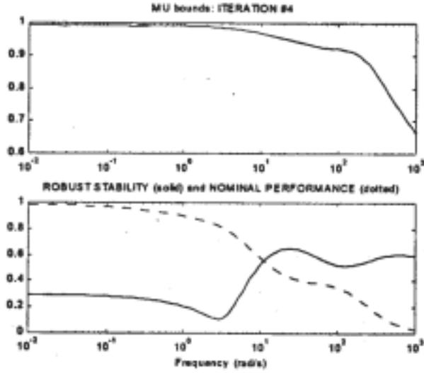
Fig. 6. Robust stability and nominal performance after the D-K iteration
