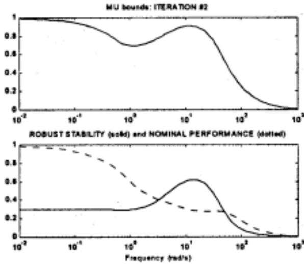
Fig. 10. Robust stability and nominal performance after the D-K iteration
