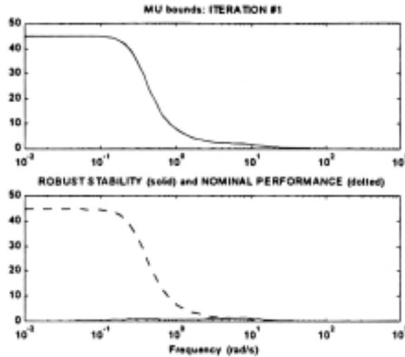
Fig. 5. Robust stability and nominal performance with  $H_\infty$  controller
