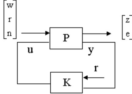
Fig. 2. Generalized closed-loop structure
