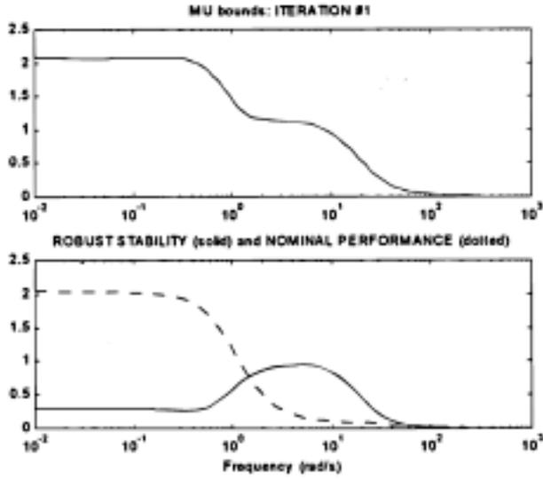
Fig. 9. Robust stability and nominal performance with  $H_\infty$  controller
