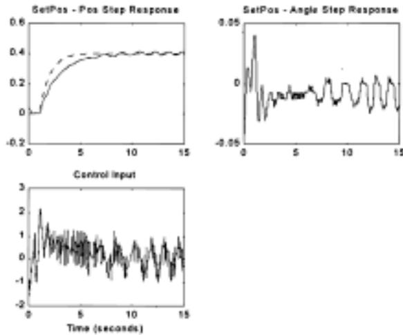
Fig. 12. Step responses of the position and of the angle with control input in real situation
