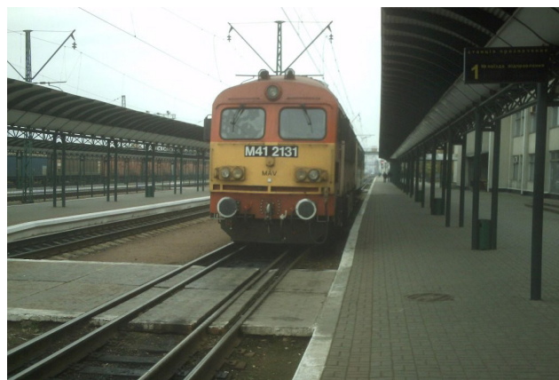
Fig. 5 The dual gauge line at the Chop station (Ukraine) (Hibberd, 2006)
