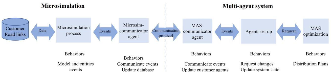
Fig. 1 Architecture for integrating multi-agent system and microsimulation
