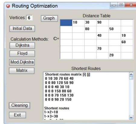
Fig. 2 Window of subprogram for determining the optimal routes
