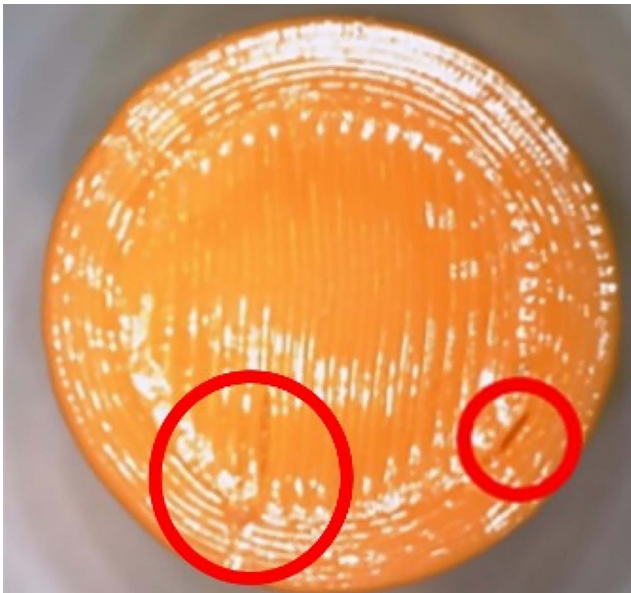
Fig. 13 Printing error; note: 0.4 mm layer thickness, vertical orientation
