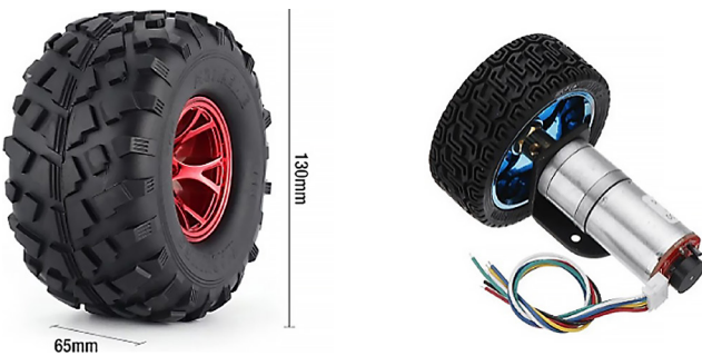
Fig. 12 Wheel and electric motor (Machifit 25GA370 DC 12V, Speed: 190 rpm, Torque 5,0 kgf.cm)
