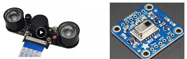
Fig. 14 Raspberry Pi Night Vision Fisheye Camera 5MP, IR thermal camera (Panasonic, Temperature range: 0-80 °C, 8x8 sensor matrix)
