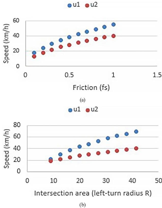
**Fig. 3** The relationship between the traversing speed with the (a) friction coefficient, and (b) area of the intersection
