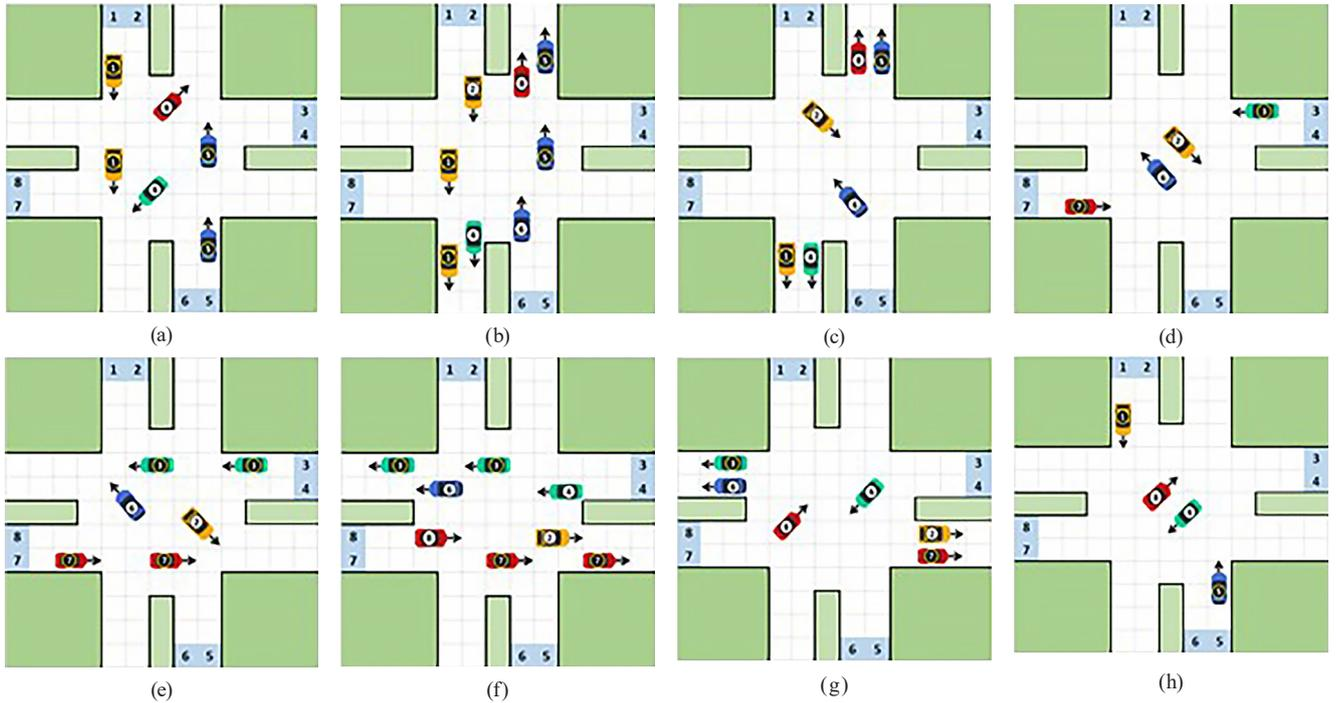
Fig. 1 Sequence of vehicle movements at the intersection by the proposed the protocol
