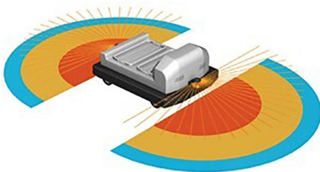
Fig. 3 Lidar and sensors on a PMV (Hokuyo, 2024)
