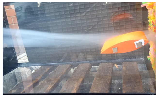
Fig. 14 The vortex is made visible with smoke
