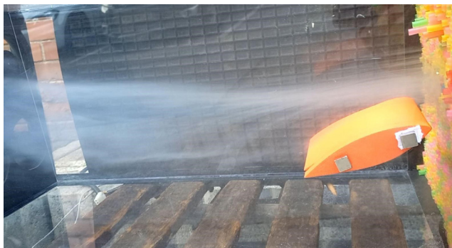
Fig. 13 3D printed model in the wind tunnel
