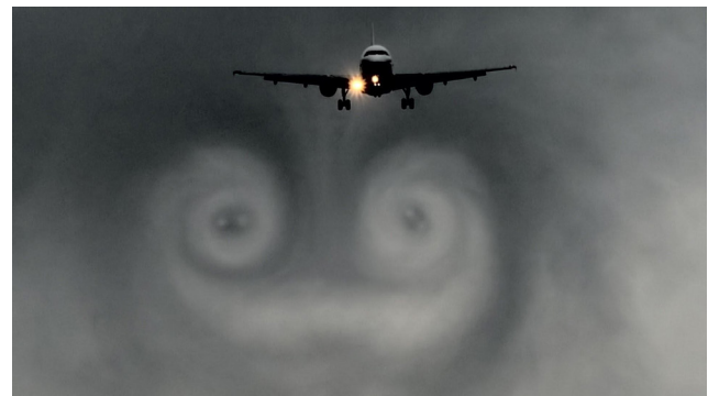
Fig. 4 Vortex behind the wingtip
