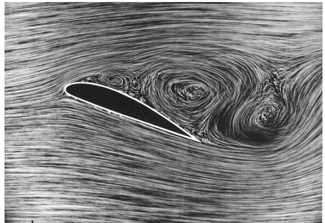
Fig. 21 Airflow at stall speed
