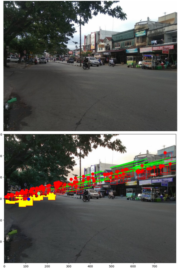
Fig. 22 Vanishing point detection results with 24 lines detected
