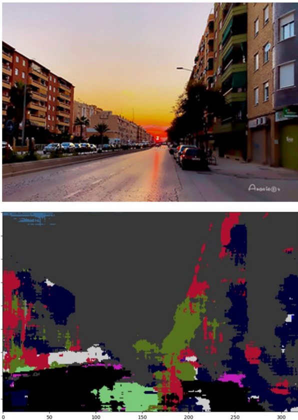
Fig. 21 Failure cases of our method in the segmentation of the road with image 320 \times 214 pixels
