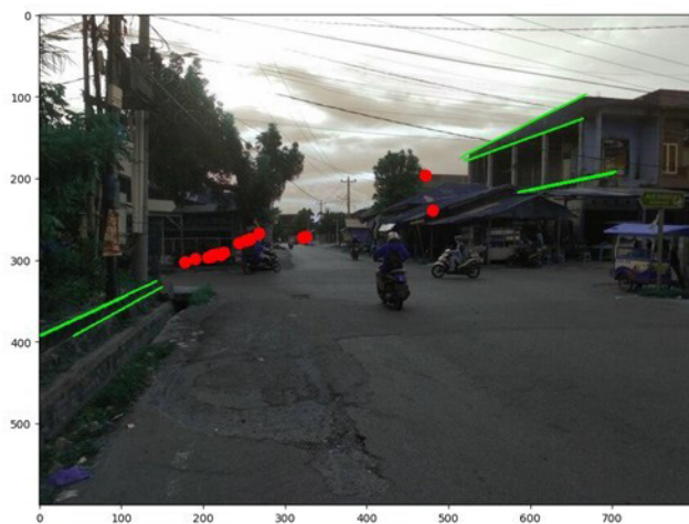
Fig. 11 Result of line detection by Hough transform and intersection point at the lower threshold value 50 and upper threshold value 100
