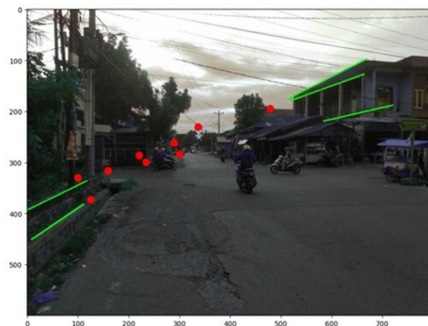
Fig. 13 Result of line detection by Hough transform and intersection point at the lower threshold value 70 and upper threshold value 100
