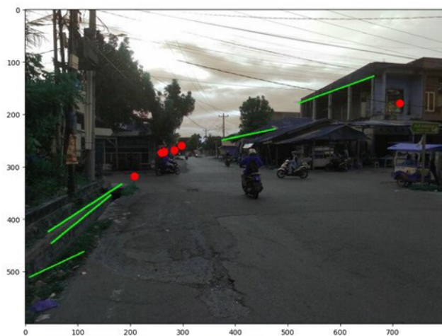
Fig. 12 Result of line detection by Hough transform and intersection point at the lower threshold value 60 and upper threshold value 100
