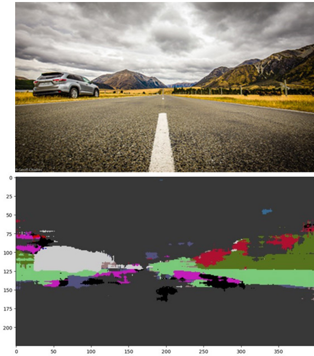
Fig. 20 Failure cases of our method in the segmentation of the road with image 400 \times 225 pixels
