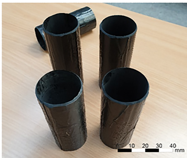
Fig. 1 The prepared composite tube specimens. The trigger geometry facing upwards with a ~30° semi-apical angle
