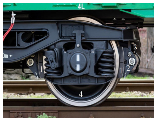
Fig. 1 The arrangement of a conventional brake system of a freight wagon (Appoh et al., 2021)
