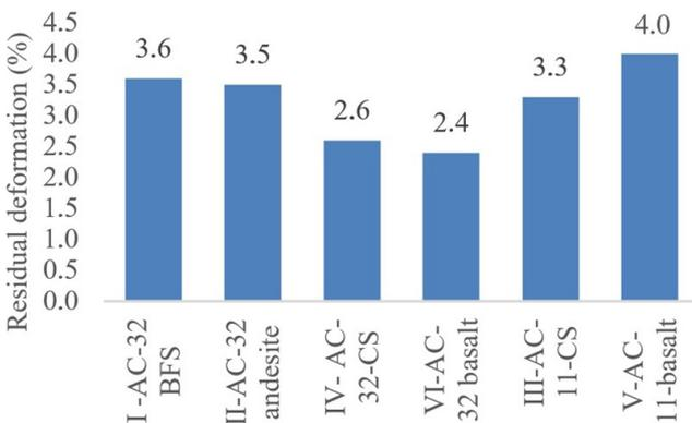
**Fig. 2** Residual deformation of reference and slag asphalts
