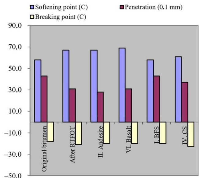
Fig. 7 Properties of recovered bitumen
