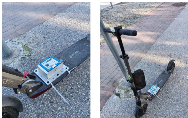
Fig. 2 E-scooter with measurement device
