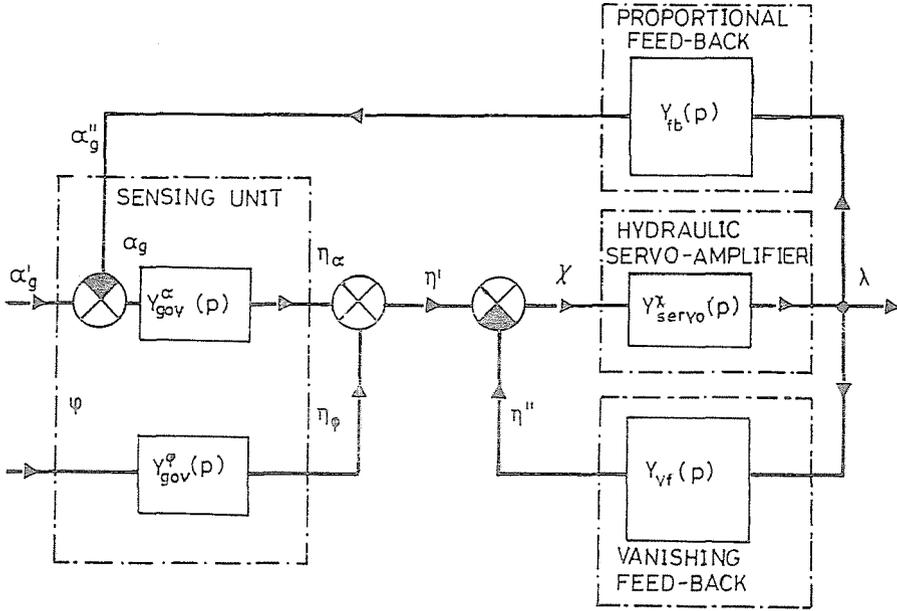
Fig. 3. Block diagram of a PI-type hydraulic universal speed governor
