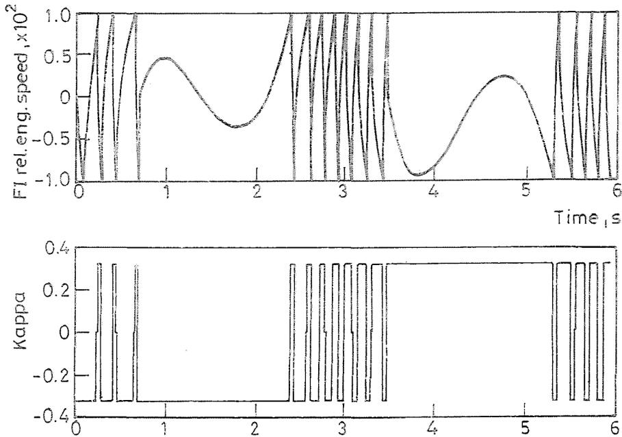
Fig. 16. Time history of  $\varphi$  and  $\kappa$ , applying  $\kappa = -0.325$  limit
