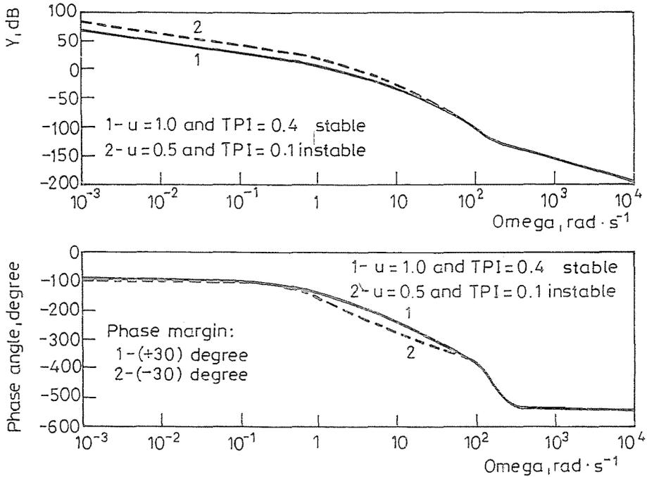
Fig. 14. Bode diagram of the open control loop
