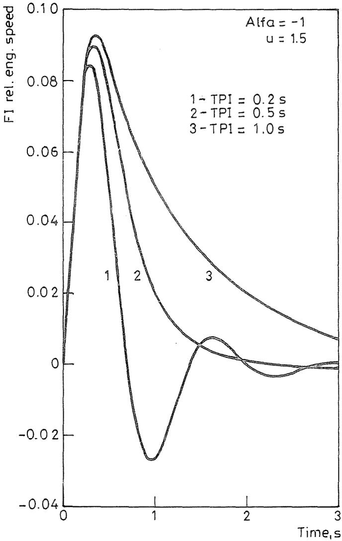
Fig. 11. Step responses at various pairs of  $u$  and  $T_{PI}$
