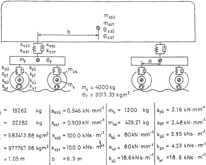
Fig. 10. Lumped parameter vertical in-plane dynamical model of the vehicle
