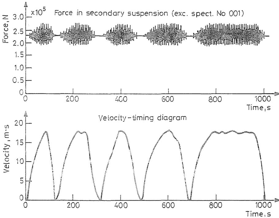
Fig. 14. Time history of vertical forces transmitted by the secondary suspension system
