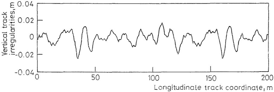
Fig. 9. Realization function of vertical track irregularities generated from spectral density function shown in Fig. 8
