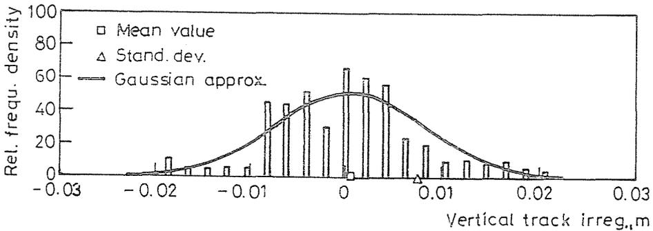
Fig. 15. Relative frequency density histogram of the vertical track irregularities
