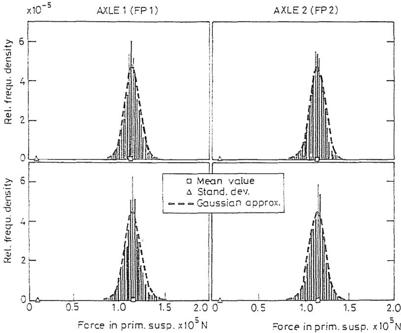
Fig. 18. Relative frequency density histograms of the vertical forces transmitted through the primary suspension system
