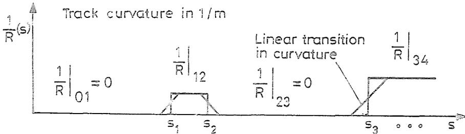
Fig. 4. Track curvature function vs. track arc length
