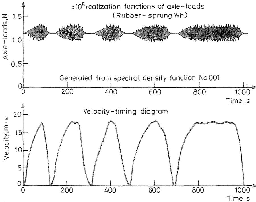
Fig. 12. Time history of the dynamic axle loads in the rubber sprung wheelsets
