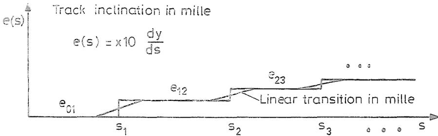
Fig. 3. Track inclination function vs. track arc length
