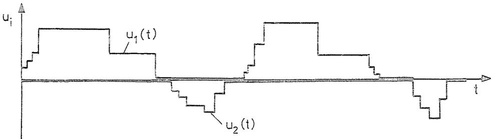
Fig. 5. Drive and brake control functions vs. time
