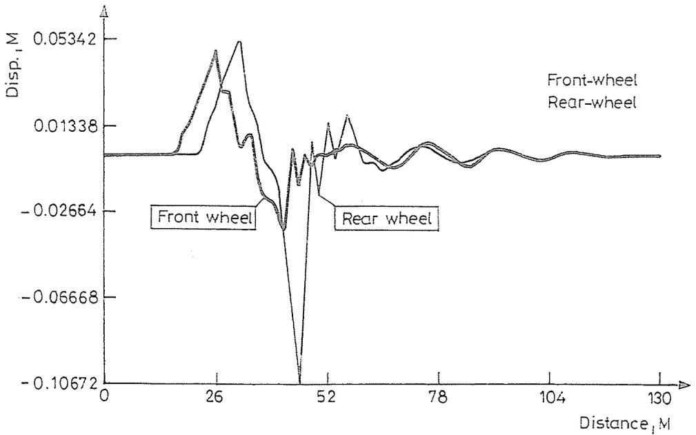
Fig. 15. Lateral motion of the right hand side wheels
