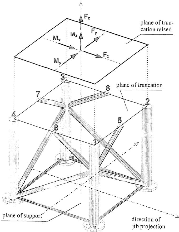
Fig. 2. Forces and moments in the cutting plane
