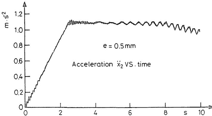
Fig. 4. Blown up section of the perturbational solution
