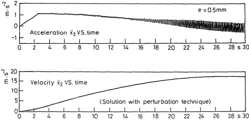
Fig. 3. Vibration form obtained by perturbational techniques
