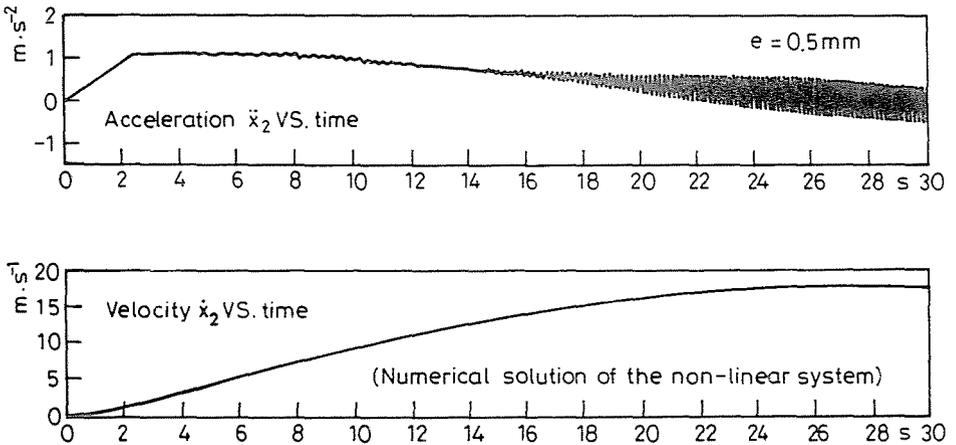
Fig. 2. Vibration form obtained by direct numerical solution
