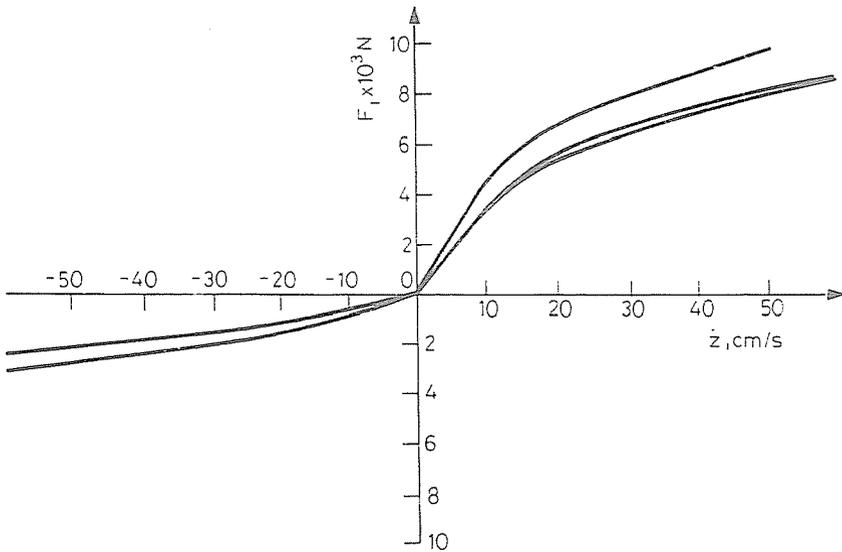
Fig. 9. Solution with swinging lever  $\alpha = 30^\circ$ , amplitude of the periodic excitation = 10 cm, angular frequency  $\omega = 6$  rad/s.
