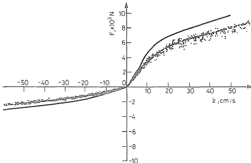
Fig. 10. Solution with rigid axle,  $\alpha = 30^\circ$ , the vehicle runs on earth road, standard deviation of the road profile = 6 cm, velocity of the vehicle = 45 km/h.
