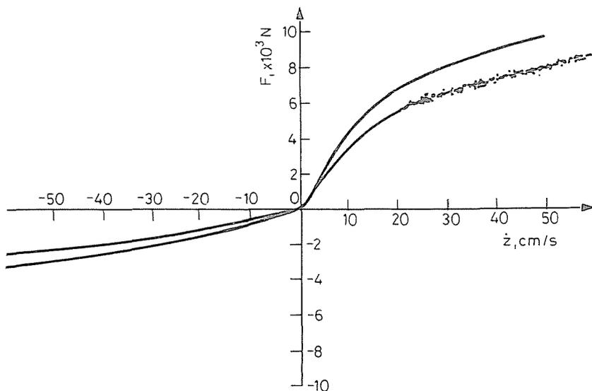
Fig. 11. Solution with swinging arm,  $\alpha = 30^\circ$ , the vehicle runs on earth road, standard deviation of the road profile = 6 cm, velocity of the vehicle = 45 km/h.
