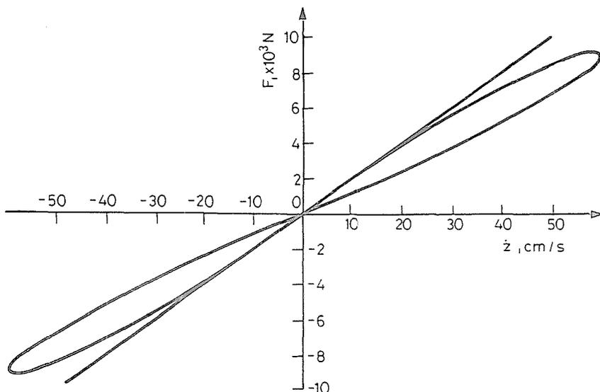
Fig. 1. Linear damping characteristic, swinging lever suspension  $r = 20$  cm,  $\alpha_0 = 30^\circ$ , amplitude of the periodic excitation = 10 cm, its angular frequency  $\omega = 6$  rad/s.
