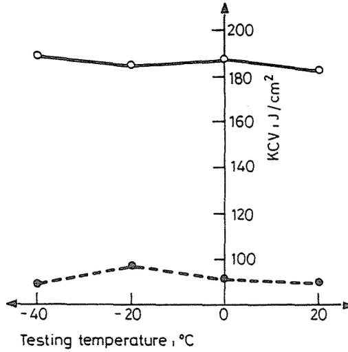
Fig. 2. Development of energy to failure in the case of specimens subject to impact test in deformation direction and perpendicular to it, respectively
