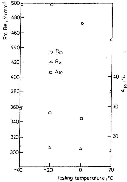
Fig. 5. Effect of rolling direction in the case of welded specimens
