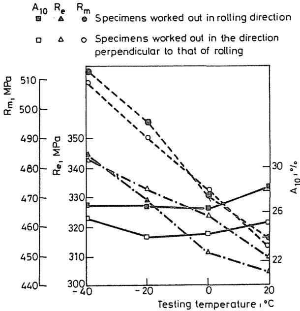
Fig. 1. Static material characteristics of specimens worked out of the basic material in deformation direction and perpendicular to it
