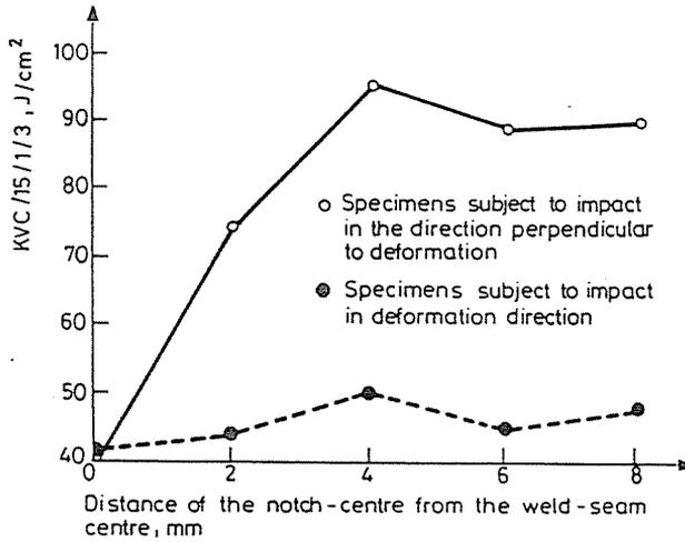
Fig. 6. Development of impact energy in the neighbourhood of welding seam
