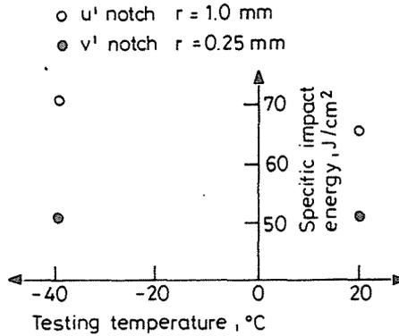
Fig. 3. Effect of chamfering the notch on the specific impact energy at different temperatures
