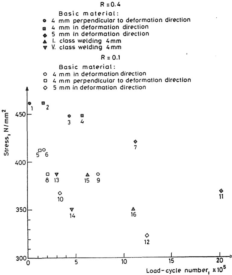
Fig. 4. Effect rolling direction on the load-cycle number to failure
