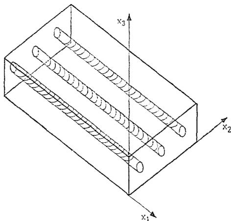
Fig. 2. Arrangement of steel reinforcement in the belt
