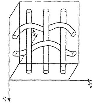
Fig. 1. Structure of the belt reinforced with carcass
