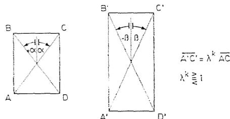
Fig. 4. Strain of the material system reinforced with diagonal cord
