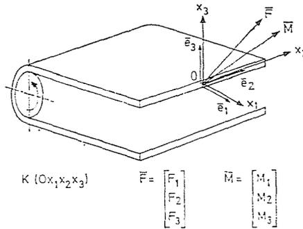
Fig. 3. Vectors  $F$ ,  $M$  representing the mechanical load of plain belt
