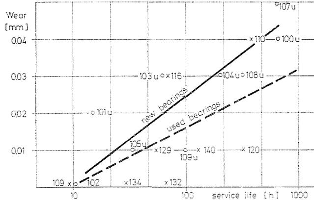
Fig. 10. Wear of taper roller bearings
