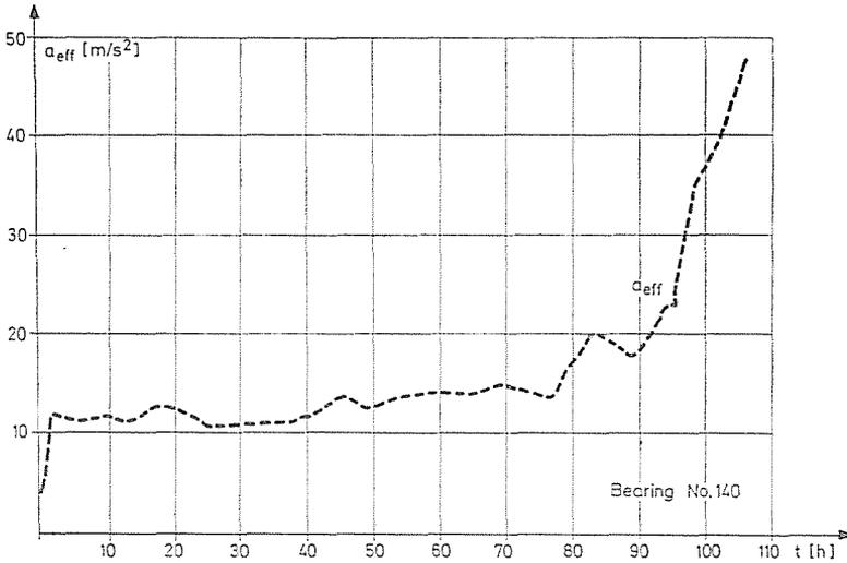
Fig. 12. Vibration intensity variation of a taper roller bearing in the service life test
