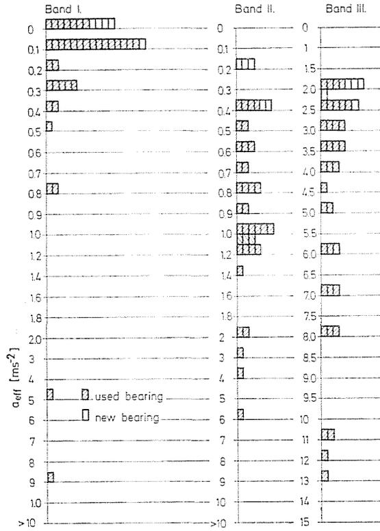
Fig. 6. Distribution of bearing vibrations between bands (type 32308)
