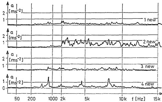
Fig. 2. Vibration spectra of new bearings
