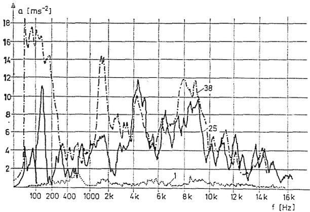
Fig. 3. Vibration spectra of used bearings
