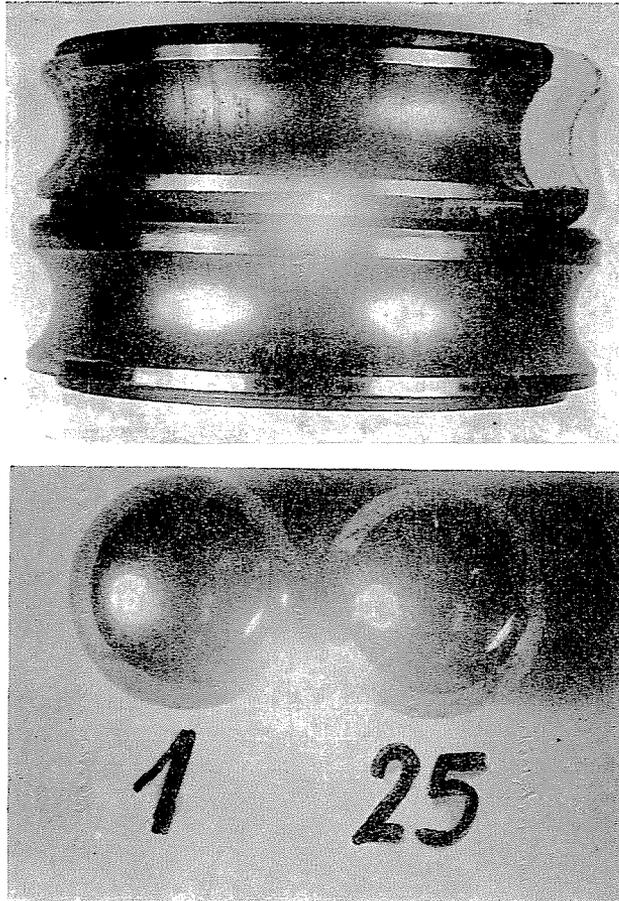
Fig. 4. Surfaces of the inner ring and of the roller element of used bearings
