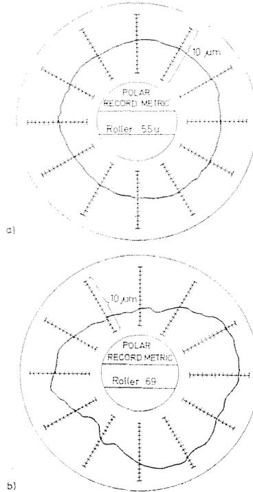
Fig. 11. Bearing roller shapes, a) new; b) used
