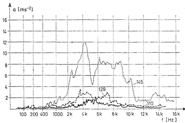
Fig. 5. Vibration spectra of new and used taper roller bearings
