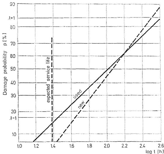
Fig. 9. Diagram of service life damage probability of new and used bearings
