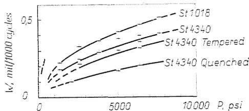
Fig. 9. Effect of specific pressure on the fretting wear. slip = 0.012 in. C = 20cps
