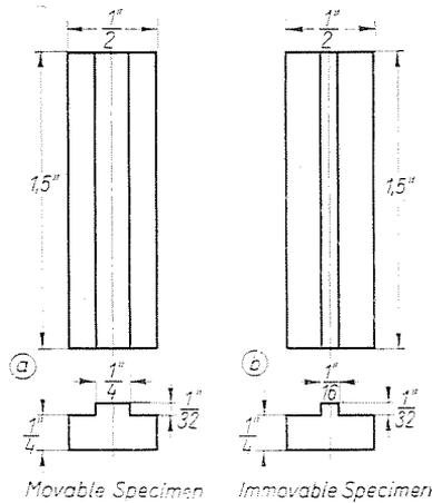
Fig. 2. Fretting specimens
