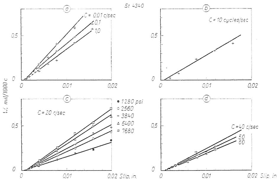
Fig. 6. Effect of amplitude (slip) on fretting wear
