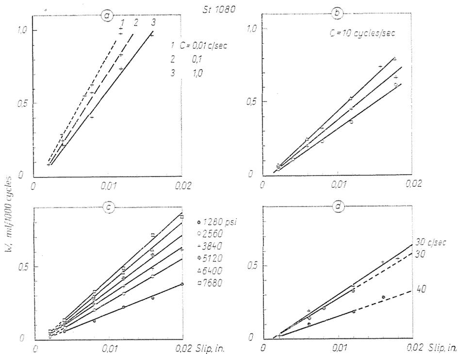
Fig. 5. Effect of amplitude (slip) on fretting wear
