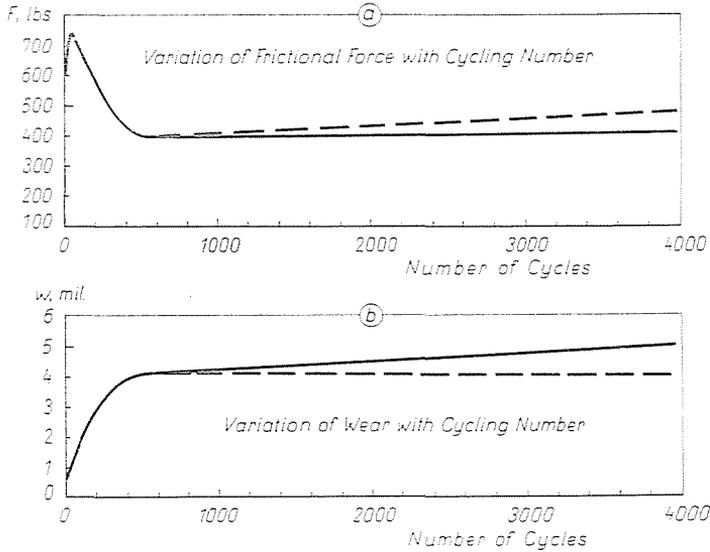
Fig. 4. Effect of duration of test on fretting 4340 steel;  $p = 6400$  psi;  $C = 20$  cps; slip = 0.012 in
