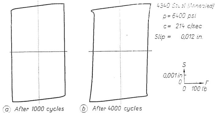
Fig. 3. Friction force ( $F$ ) and stroke ( $S$ ) diagram 4340 steel (annealed);  $p = 6400 \text{ psi}$ ;  $c = 214 \text{ cps}$ ; slip = 0.012 in
