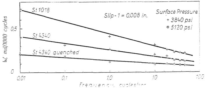
Fig. 8. The effect of frequency on fretting wear
