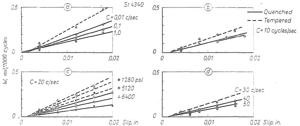
Fig. 7. Effect of amplitude (slip) on fretting wear
