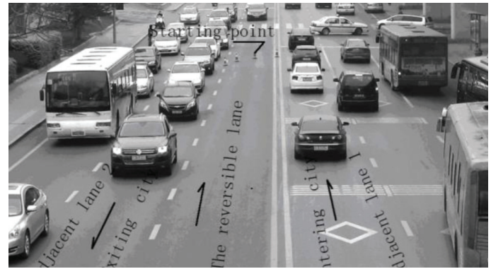
Fig. 3. The reversible lane with lower utilization ratio
