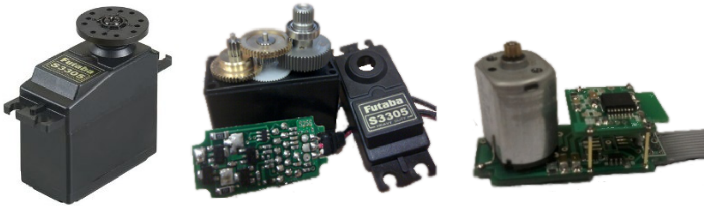
Fig. 2. Futaba S3305 COTS RC servo and the custom servo with measurement and power electronics
