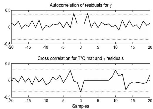
**Fig. 5** Autocorrelation and cross-correlation regarding the output density ( $\gamma$ ) and the input Temperature of the asphalt material ( $T_e\_M$ ). The residuals are widely inside the confidence interval region, indicating that all the dynamics have been captured by the model.
