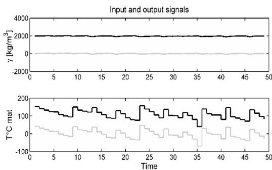
**Fig. 1** Trend of the density of the asphalt materials  $\gamma$  (top) in relationship with the Temperature of the material.
