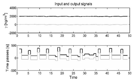
**Fig. 2** Trend of the density of the asphalt materials  $\gamma$  (top) in relationship with the elapsed time during the single pass of the roller.
