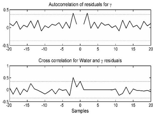
**Fig. 7** Autocorrelation and cross-correlation regarding the output density ( $\gamma$ ) and the input Water contained in the surface layer of the pavement ( $W_a$ ). Also in this case, the residuals are widely inside the confidence interval region, indicating that all the dynamics have been captured by the model.
