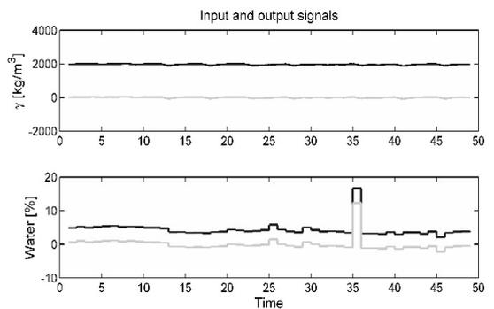
**Fig. 3** Trend of the density of the asphalt materials  $\gamma$  (top) in relationship with the water on the layer surface.
