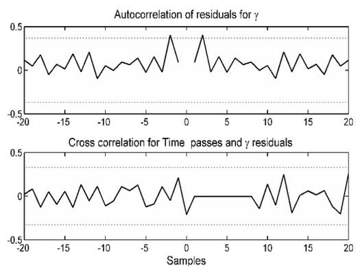
**Fig. 6** Autocorrelation and cross-correlation regarding the output density ( $\gamma$ ) and the input Elapsed time during the single pass of the roller ( $TI$ ). Also in this case, the residuals are widely inside the confidence interval region, indicating that all the dynamics have been captured by the model.
