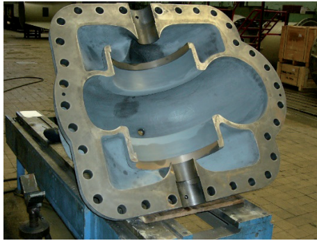
Fig. 32 Volute chamber to be prepared
