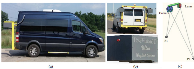
Fig. 1 Photographs of (a) DHDV exterior appearance (b) DHDV rear view with PavVision3D sensors; (c) Pavvision3D working principle
