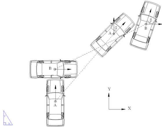
Fig. 1 Schematic diagram of vertical side collision
